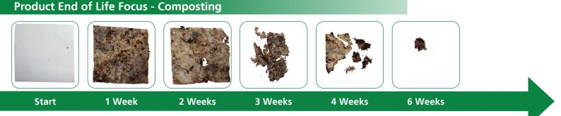
Film made from Natur-Tec<sup>®</sup> resins is fully compostable in compliance with **ASTM D6400** and **EN 13432**. Composting is the biological process of breaking up organic matter such as food, food scraps, leaves, grass trimmings, paper, bioplastics and more, resulting in biomass (nutrient rich soil amendments).
